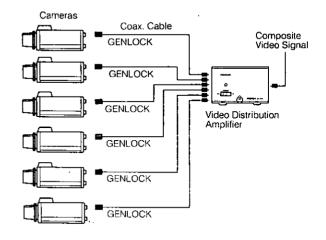
The Gen-lock Termination Switch of all cameras should be set to 75 ohm position.
