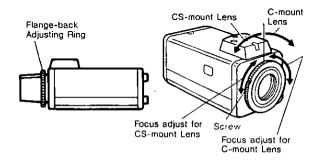
Turn the flange-back adjusting ring to the desired position.
