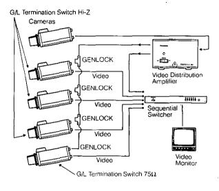
\* The Gen-lock Termination Switch of the furthest camera should be set to 75 ohm position and that of all other cameras should be set to Hi-Z position.
